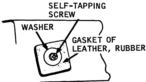
Figure 78. Pinhole-size leaks in fuel tanks.
